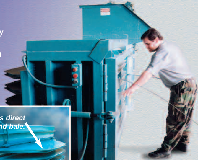
Operator inserting wire ties.
